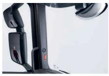
as Driver Assistant System Detection, available for the new S-Way and X-Way. This is a radar-based blind-spot monitoring system which gives visual and audible warnings in-cab for the driver
